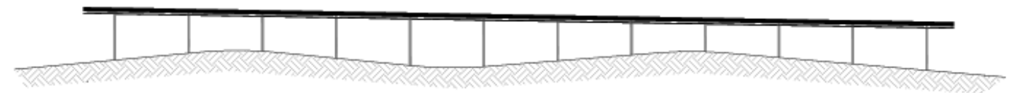
Traditional Single Axis Tracker Using increased steel pile lengths to account for ground undulations
